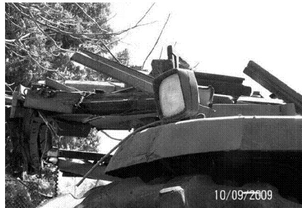
Photograph 2 – Failed ROPS, side view.
