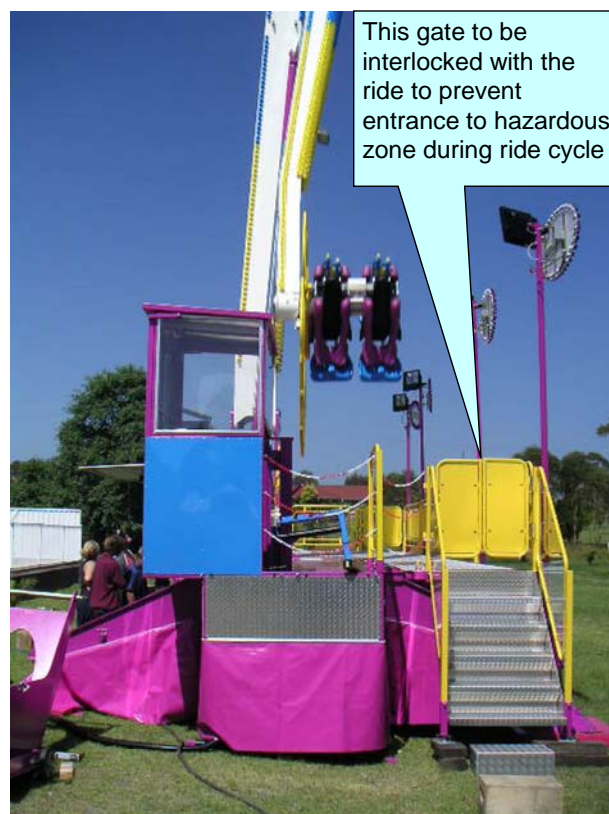
Photograph 1: View of an aerial ride showing the gates into the hazardous zone.
