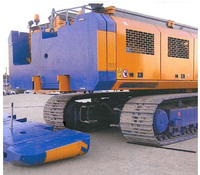
Photograph 1: rear of the drilling rig showing 10 tonne counterweight on the ground.
