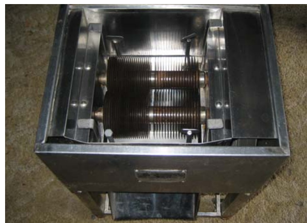
Photograph 3 – Cutting blades exposed with the feed hopper and top cover removed.
