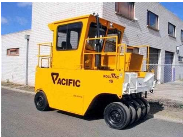
Photo 1: Showing a Pacific Roll Pac 16 tonne multi-tyred roller.
