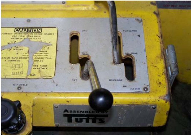
Photo 2: Showing the gear shift arrangement
