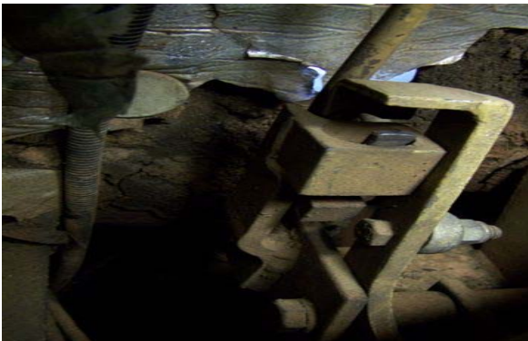
Photo 3: Showing the interlock arrangement from manufacture controlling the engagement of the forward gear shift mechanism.
