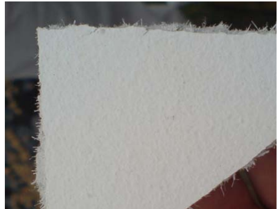
Photograph 2: Low density asbestos fibre board
