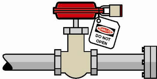
Figure 4: Open end of pipe capped. Nearest valve closed locked and tagged.
