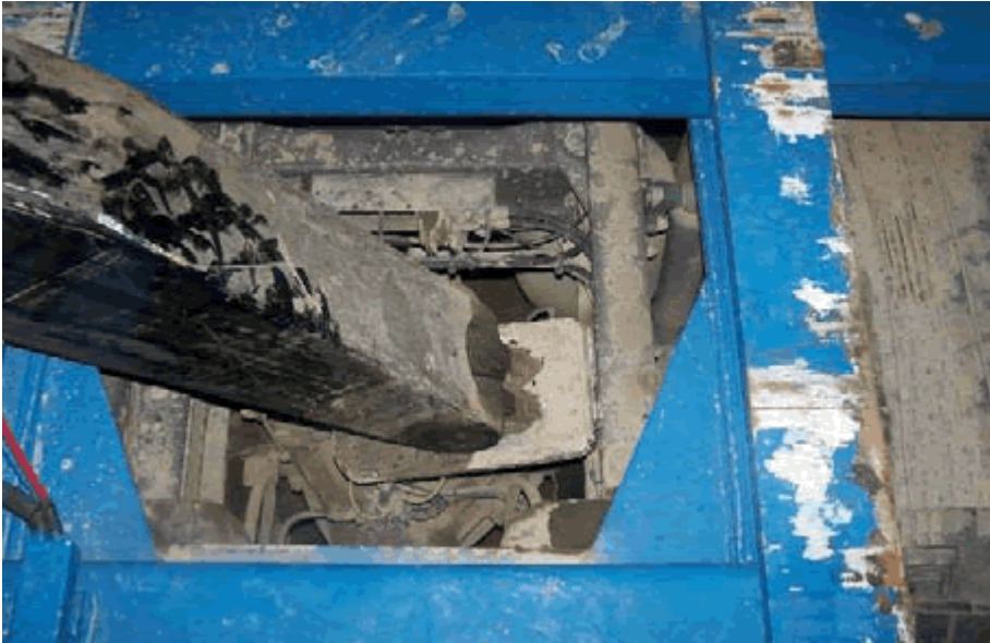
Photograph 2: Foot that has slipped off chassis
