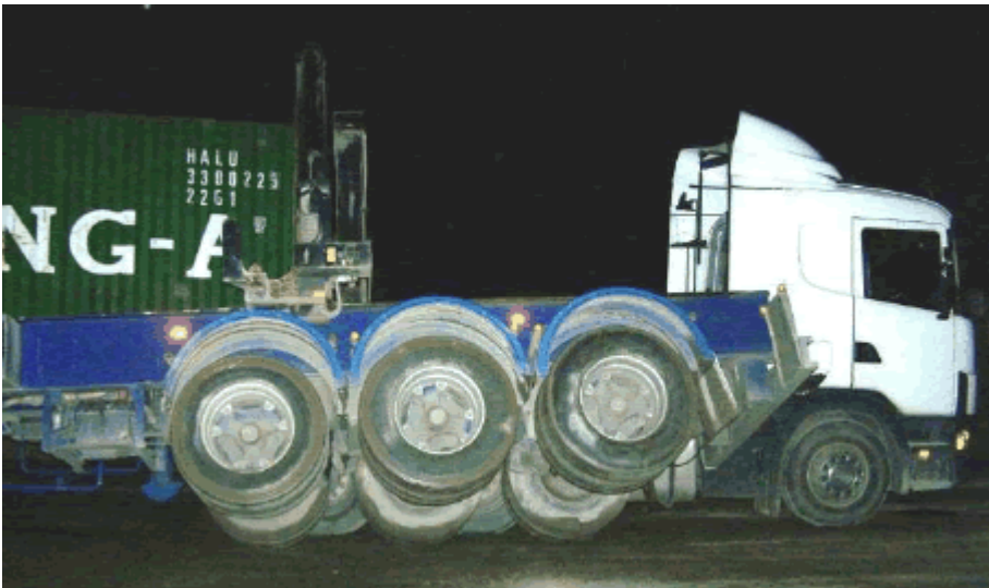
Photograph 3: Trailer tilted resulting from foot instability
