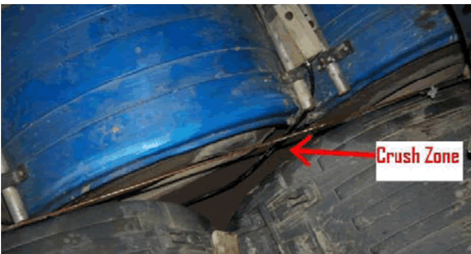
Photograph 3: Trailer tilted resulting from foot instability
