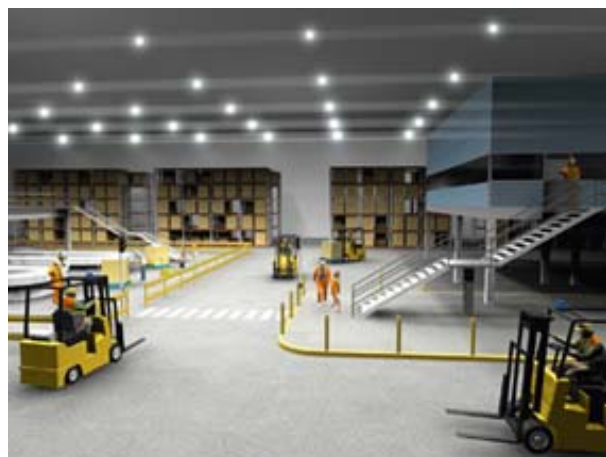
Mobile plant operated in areas where people work may cause injury through collision. Traffic control and segregation are forms of control.
