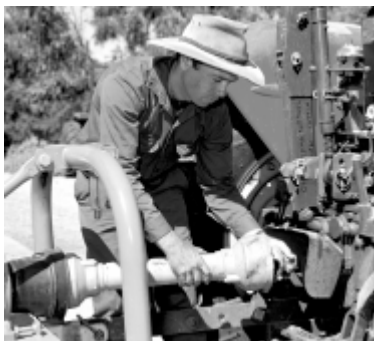
Figure 1. Tractor being fitted with PTO guard.
