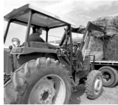
Figure 4. Tractor fitted with a FEL, specifically designed for loading/unloading hay bales.
