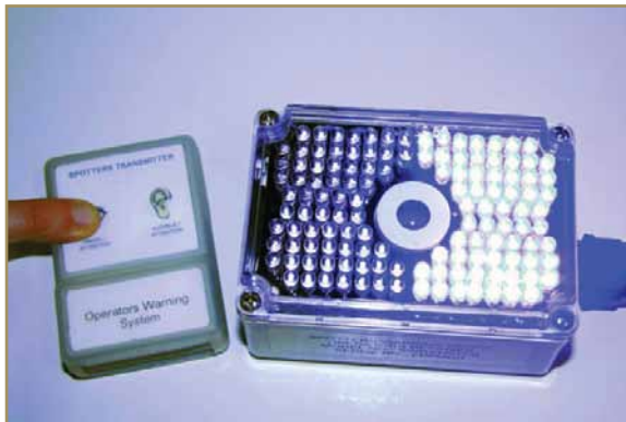
The spotter warning device with visual attention alarm armed
