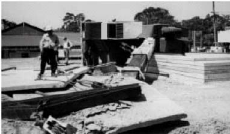
Diagram 7 – Rubber tyred pick and carry crane overturned
